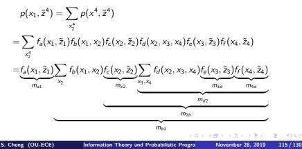
We can see from the last equation that the joint probability can be computed by combining a sequence of messages passing from a variable node *i* to a factor node  $a(m_{ia})$  and vice versa  $(m_{ai})$ . More precisely, we can write
