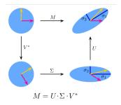
Every matrix M can be decomposed as M = UDV<sup>†</sup>, where D is diagonal and U, V are unitary. The diagonal terms in Σ are known to be the singular values
