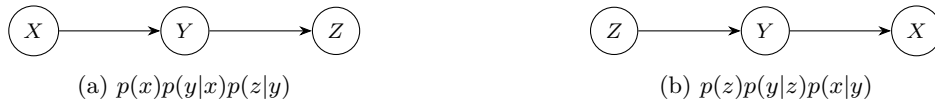
Figure 7.1: BNs for joint distribution p(x, y, z) equal to p(x)p(y|x)p(z|y) and p(z)p(y|z)p(x|y) . Despite the difference in arrow direction, the two BNs represent the same underlying probability structure.
