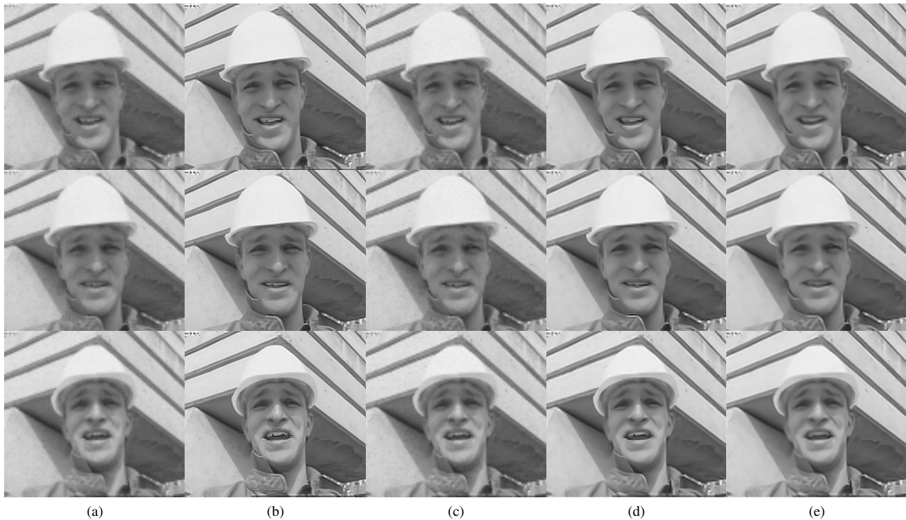
Fig. 6: Results for the 8 th , 13 th and 23 th frame from the “Foreman” sequence. From Left column to Right column: LR frame; GNL-Means [6]; Lanczos interpolation [40]; result of the proposed SCoBeP-NLM; result of the proposed SCoBeP-SR. Also, the PSNR values for all the frames are shown in Fig. 7(b).
