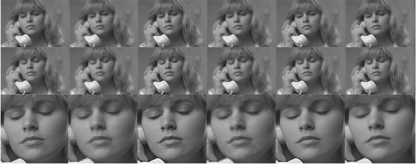
Fig. 9: Video super resolution for Suzie sequence: (frame 28 and 18 with the resolution ratio 3, PSNR in brackets). From Left column to Right column: Ground truth; LR frame; GNL-Means [6] [PSNR: 29.87 - 29.86]; Lanczos interpolation [40] [PSNR: 29.41 - 29.27]; SCoBeP-NLM [PSNR: 30.95 - 30.75]; SCoBeP-SR [PSNR: 30.55 - 30.71].
