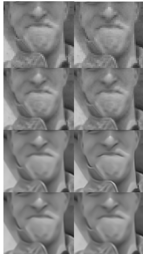
Fig. 13: Video super resolution for Foreman sequence with noise: we added synthetic additive white Gaussian noise (AWGN) to the input LR sequence, with the noise level \sigma_n = 1.20 (left) and \sigma_n = 2.00 (right). From top to bottom column: Noisy LR; 3-D ISKR [9]; SCoBeP-NLM; SCoBeP-SR.
